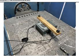
Mechanical Shock Test: ±Y axis
