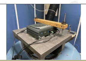
Mechanical Shock Test: ±Z axis
